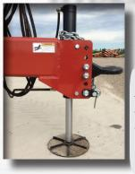
Provides quick, easy disconnection from tractor. Lifts vertically without moving machine backward and forward. Designed with less moving parts for a simpler more reliable operation.
