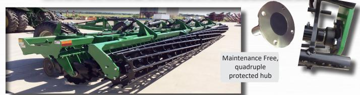
**CAGE ROLLER** (standard): works best in dry, non-sticky soil conditions. The cage design ensures disintegration of any clumps, provides an even seedbed and moderate compaction.
