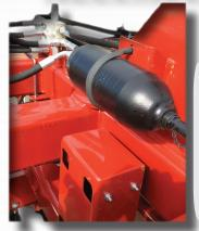
The accumulator is used in conjuction with a cross over relief valve to protect the wing cylinders from damage. Helps prevent damage by overextending cylinders or if the float position is forgotten to be put in place before use.
