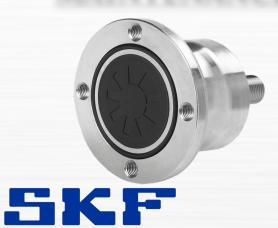
Relubrication-free: integrated solution increases farm productivity. Suitable for virtually any agricultural implement arm, the SKF Agri Hub for tillage discs is a robust, easy fit hub sealing solution. The unit features a flanged outer ring that is predrilled and tapped to accommodate a disc. A stationary inner ring fitted with a threaded stub shaft helps ensure fast, easy mounting.
